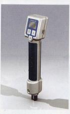
Flash 3036 tests steel's passivity, producing an immediate pass/fail signal and displaying the measurement in millivolts. For more information about this year's INTERPHEX trade show, go to page 34.
